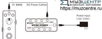
If the input polarity of the electrical device is ⊖€⊕, please connect polarity reversal cable to the DC power cable, then connect the device.
